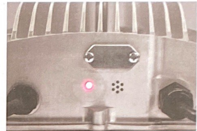
Red LED light indicating absence of AC voltage or fault code
